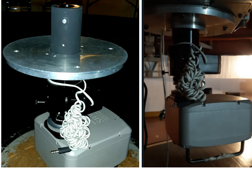
Fig. 15. Left: Mount of the WeDoWo holder inside the structure that attach the optical CCD to the telescope. The design takes into consideration this structure. Right: CCD structure properly attached to the telescope, the WeDoWo holder is already inside.
