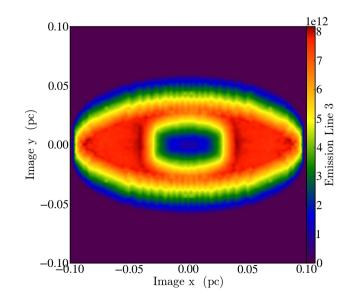
example of a simple flat disk, with uniform density of 4000 cm<sup>-3</sup>, ionized by the central black body with temperature of 75 000 K
