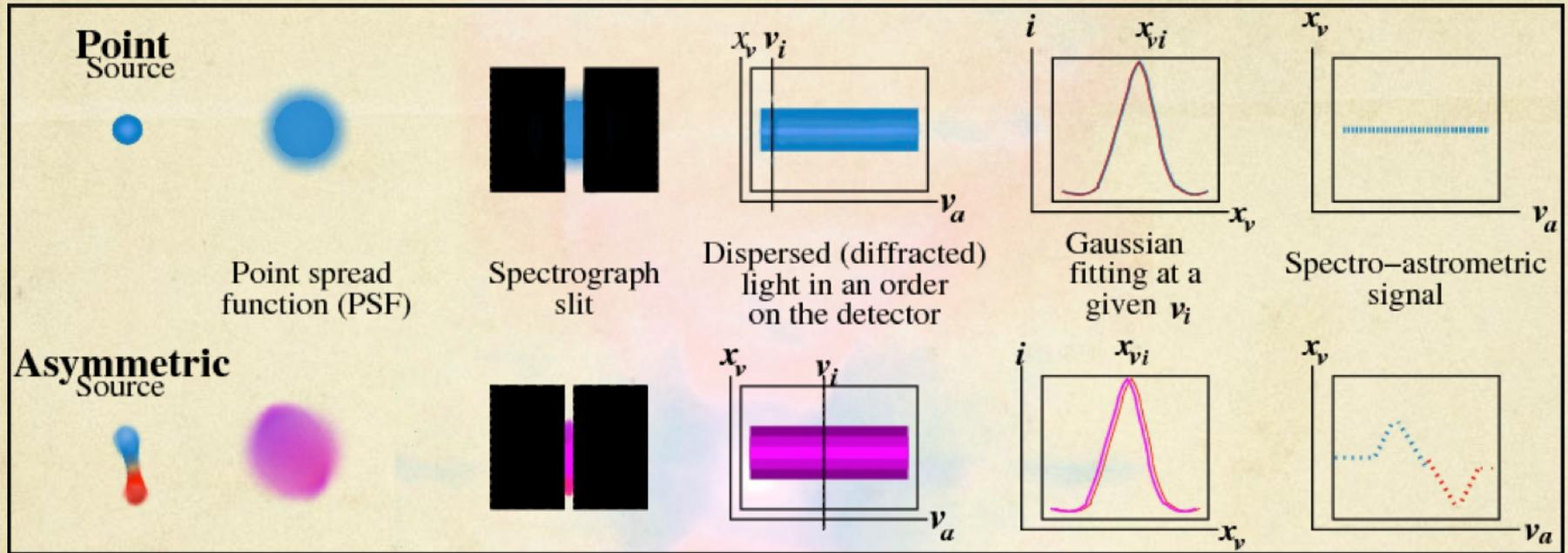
Sketch of the SA technique for a point source and an asymmetric source, both blurred by the seeing (adapted from Whelan et al. 2008).
