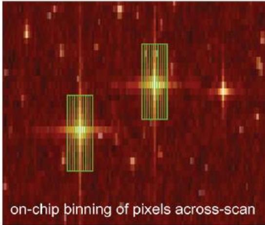
**Figure 3.** Simulated CCD image of a stellar field as observed by Gaia astrometric instrument. Credits: Gaia DPAC-CU2.
