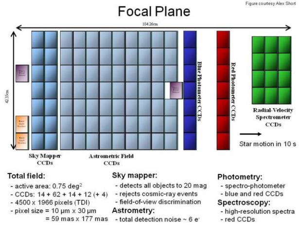
Figure 2. Gaia focal plane showing CCD properties and several fields corresponding to each of the instruments.
