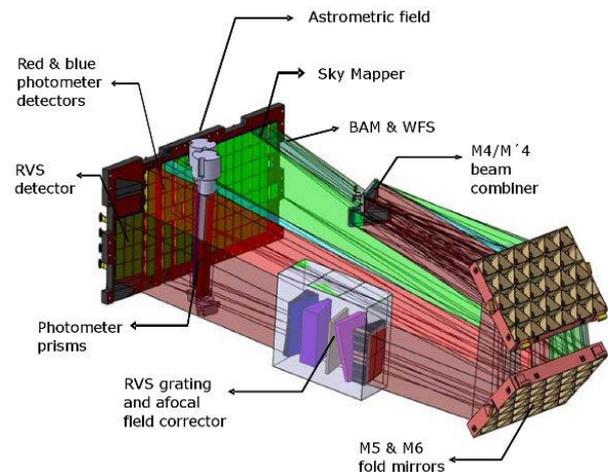
**Figure 1.** Gaia instruments and the common focal plane.
