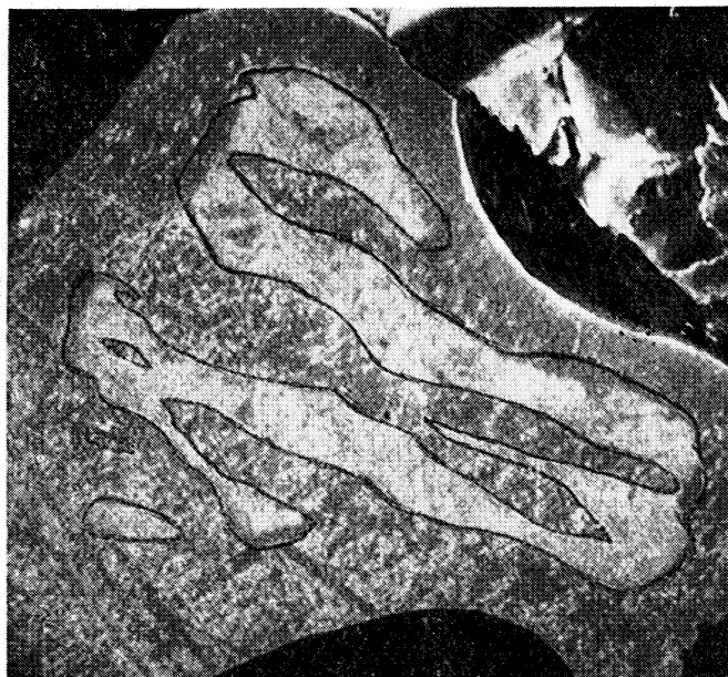
FIG. 4. Iron-nickel blebs in the core of an orthopyroxene crystal. Nearly square holes are visible ; on the left corners, the pyroxene rim is compact \times 3\ 000 .
