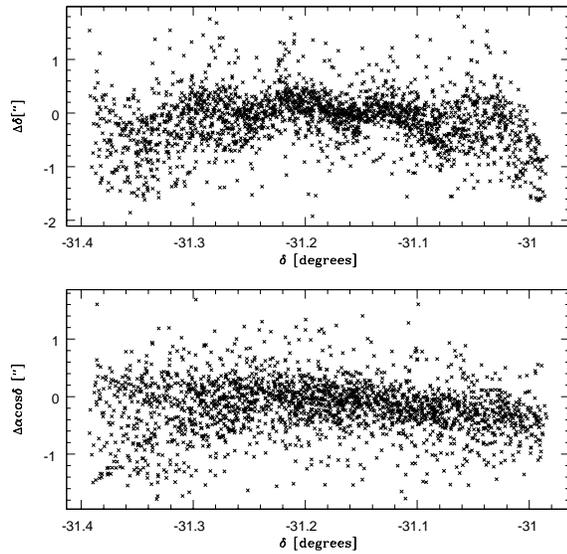
Fig. 5. Differences between positions measured with the CCD and the ones given in USNO-A2 against declination.
