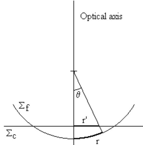
Fig. 7. Field curvature model for the pattern in Fig. 6.  $\Sigma_f$  is the focal surface and  $\Sigma_c$  is the CCD surface.  $r$  and  $r'$  are the radial coordinates on the focal surface and the one measured on the CCD, respectively.
