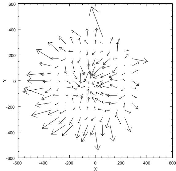
Fig. 6. Differences between CCD-based positions and USNO-A2 averaged within a grid of square cells  $\approx 60$  pixels on a side. The coordinates  $x$  and  $y$  of grid cells on the frame are given in pixels. Vectors have been enlarged 250 times, so the biggest ones represent approximately  $1''$  ( $\approx 1.2$  pixel).
