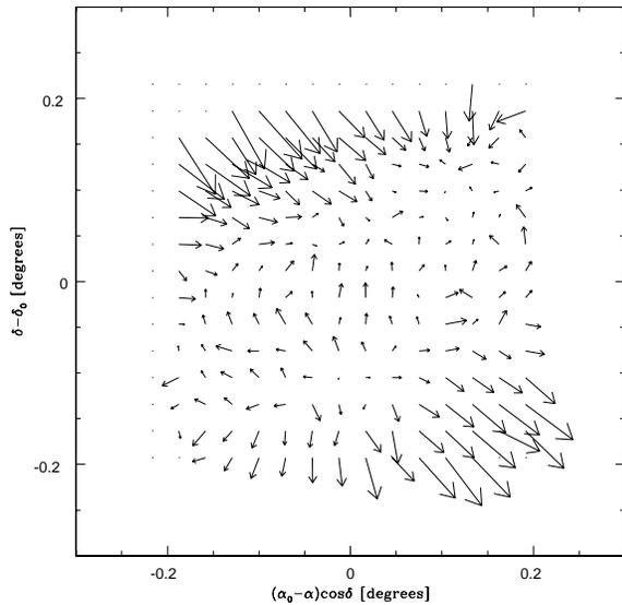
Fig. 11. Differences between CCD-based positions and USNO-A2 averaged within a grid of square cells 1'.7 on a side.  $(\alpha, \delta)$  are coordinates of grid cells and  $(\alpha_0, \delta_0)$  is the approximate center of the field. Vectors have been enlarged 180 times, so the biggest ones represent approximately 1''.5.
