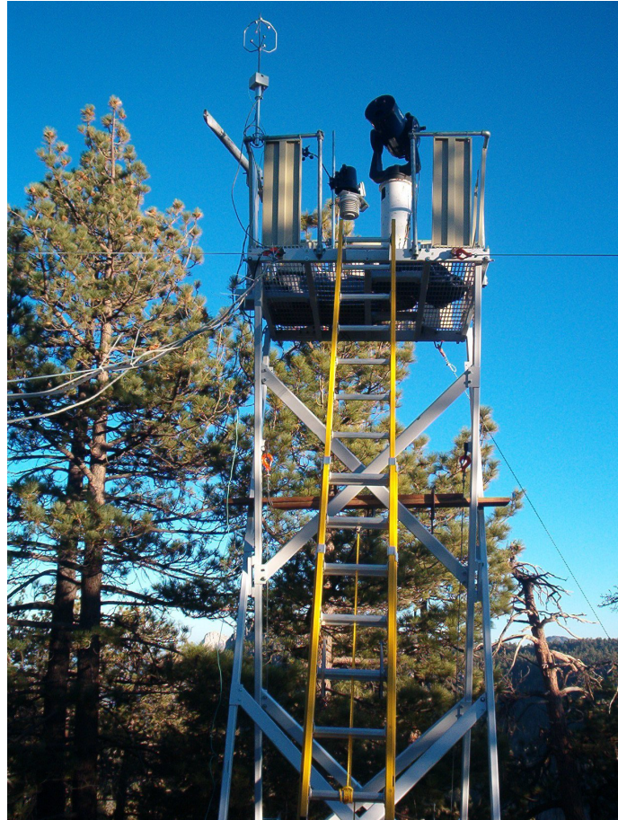
Fig. 3. Transportable tower at the Camino Viejo site. The RoboDIMM unit, the Davis meteorological station and the Metek ultrasonic anemometer are clearly visible.
