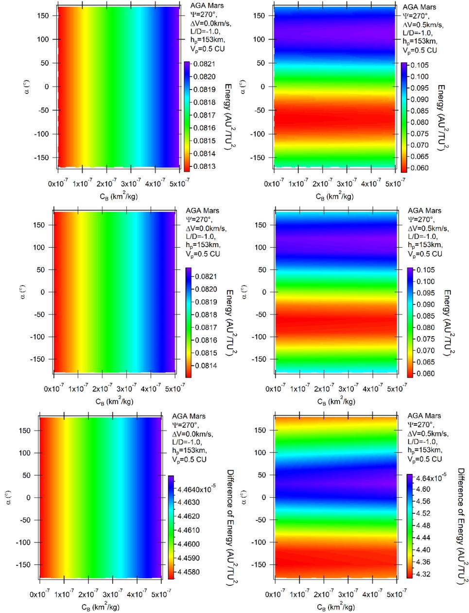
Fig. 6. Variation of energy per unit of mass as a function of the angle of attack for AGA with  $L/D = -1$  and  $\psi = 270^\circ$  for retrograde (above) and direct (middle) orbits. The differences between direct and retrograde orbits are shown in the bottom part of the figure. The color figure can be viewed online.
