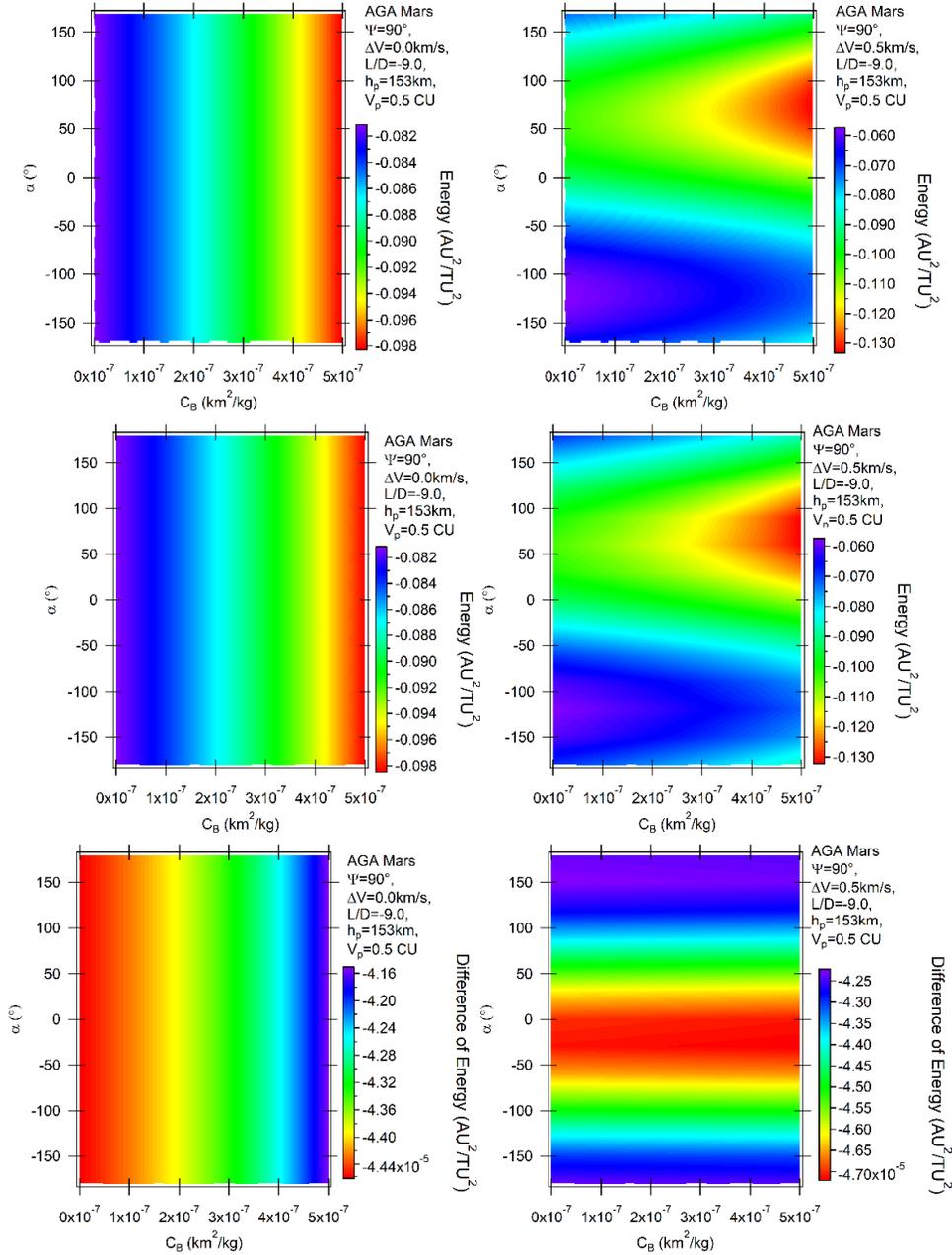
Fig. 5. Variation of energy per unit of mass as a function of the angle of attack for AGA with  $L/D = -9$  and  $\psi = 90^\circ$  for retrograde (above) and direct (middle) orbits. The differences between direct and retrograde orbits are shown in the bottom part of the figure. The color figure can be viewed online.
