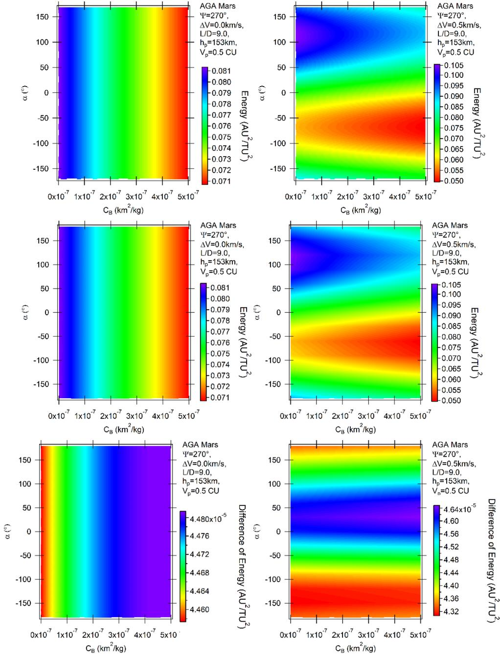
Fig. 9. Variation of energy per unit of mass as a function of the angle of attack for AGA with  $L/D = 9$  and  $\psi = 270^\circ$  for retrograde (above) and direct (middle) orbits. The differences between direct and retrograde orbits are shown in the bottom part of the figure. The color figure can be viewed online.
