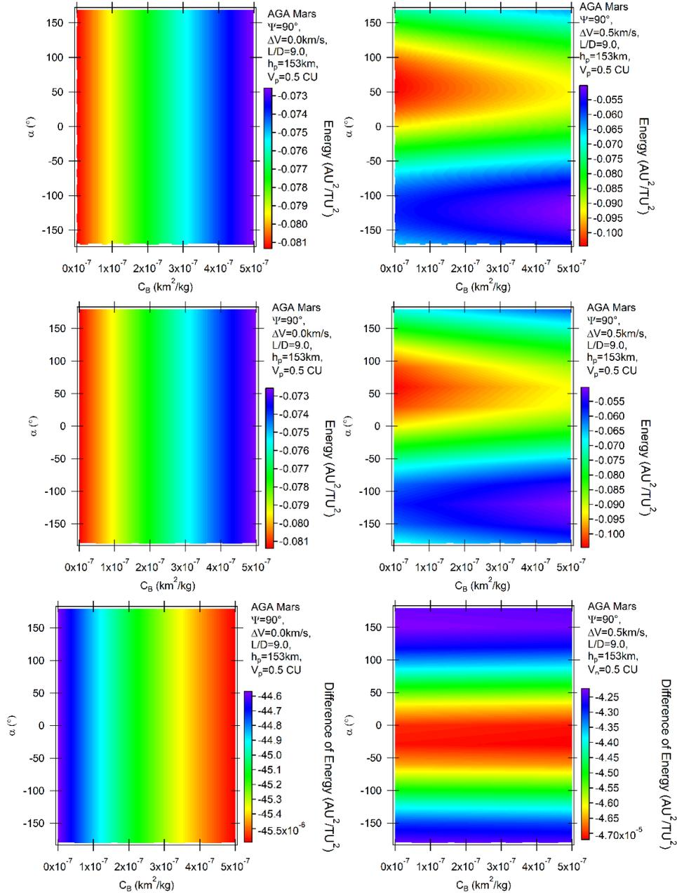
Fig. 3. Variation of energy per unit of mass as a function of the angle of attack for AGA with  $L/D = 9$  and  $\psi = 90^\circ$  for retrograde (above) and direct (middle) orbits. The difference between direct and retrograde orbits are shown in the bottom part of the figure. The color figure can be viewed online.
