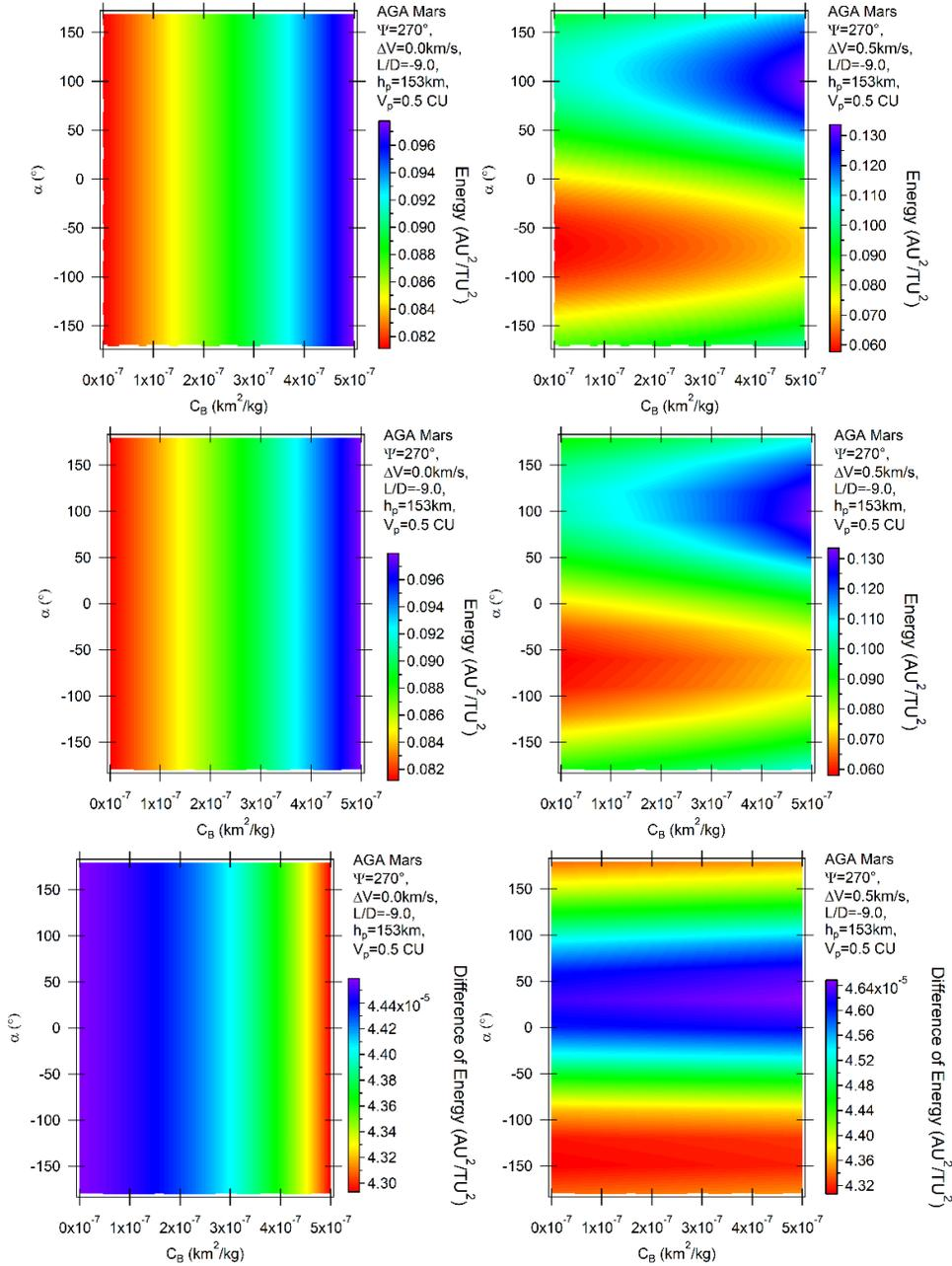
Fig. 7. Variation of energy per unit of mass as a function of the angle of attack for AGA with  $L/D = -9$  and  $\psi = 270^\circ$  for retrograde (above) and direct (middle) orbits. The differences between direct and retrograde orbits are shown in the bottom part of the figure. The color figure can be viewed online.
