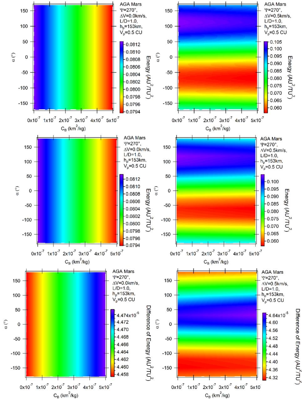
Fig. 8. Variation of energy per unit of mass as a function of the angle of attack for AGA with  $L/D = 1$  and  $\psi = 270^\circ$  for retrograde (above) and direct (middle) orbits. The differences between direct and retrograde orbits are shown in the bottom part of the figure. The color figure can be viewed online.
