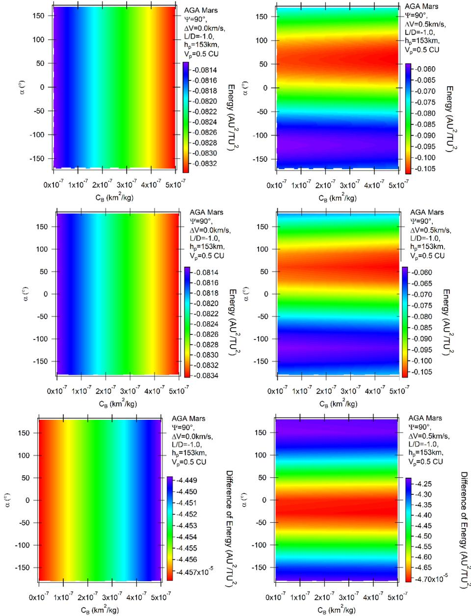
Fig. 4. Variation of energy per unit of mass as a function of the angle of attack for AGA with  $L/D = -1$  and  $\psi = 90^\circ$  for retrograde (above) and direct (middle) orbits. The differences between direct and retrograde orbits are shown in the bottom part of the figure. The color figure can be viewed online.
