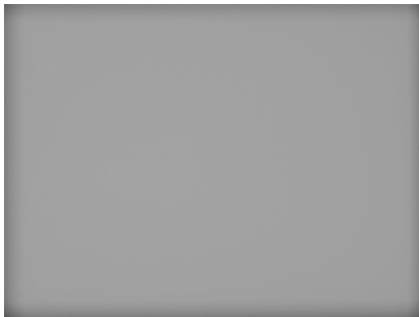
Fig. 3. Flat field image. Vignetting of the f/3 beam is caused by the rectangular frame of the mechanical shutter in front of the sensor.
