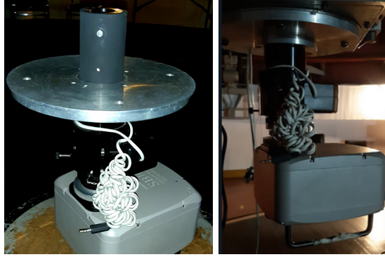
Fig. 15. Left: Mount of the WeDoWo holder inside the structure that attaches the optical CCD to the telescope. The design takes into consideration this structure. Right: CCD structure properly attached to the telescope, the WeDoWo holder is already inside. The color figure can be viewed online.
