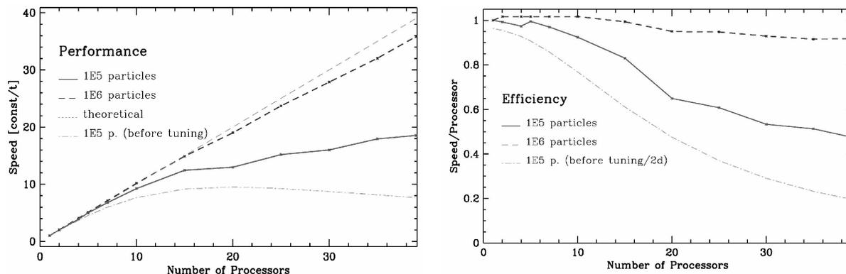
Fig. 2. Speed increase and efficiency per processor of our radiation transport code for various sizes of photon packages using PVM on our local Beowulf cluster for a configuration similar to those used in Figure 1. We used a grid of 510 radial and 120 angular coordinates. The line labeled ‘before tuning’ corresponds to the same code without the use of multi-casting and without using the option for fast communications between processors of the same family.
