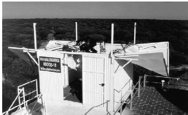
Fig. 1. BOOTES-1B dome housing one of the 30 cm Schmidt–Cassegrain telescopes and a few of the WFCs at the Centro de Experimentación del Arenosillo, in Mazagón, Huelva, Spain.
