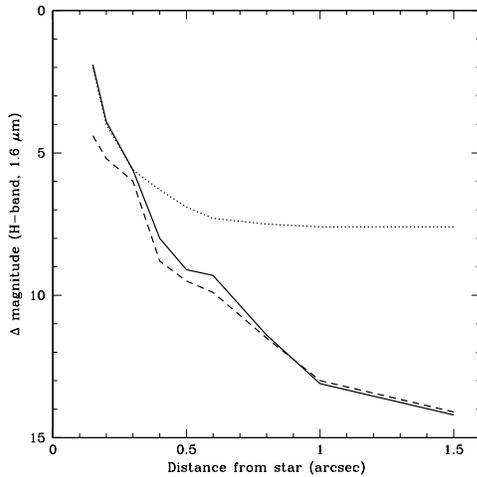
Fig. 1. Comparison of contrast sensitivities for two AO systems. Solid line: 5 sigma, 5 min, Gemini/Hokupa'a,  $V = 7$ , G2 V; Dotted line: 5 sigma, 30 min, Gemini/Hokupa'a,  $I = 13$ , M6 V; Dashed line: 5 sigma, 5 min, Keck/AO,  $V = 6$ , G2 V.
