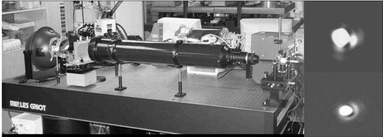
Fig. 7. Star test in double pass to measure the PSF degradation. The light goes from right to left, and is returned back by a flat mirror just next to the integrating sphere (not used in this test). On the right of the telescope a splitter cube feeds the light (diode laser beam with a spatial filter) and sends the returned beam to a microscope with a CCD. Right: PSF images before grating (down) and with the grating (up).
