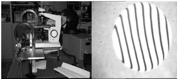
Fig. 5. Left, the assembly to measure the curvatures of the fused silica lens. On the right the interferogram supplied by INAOE for the concave surface.
