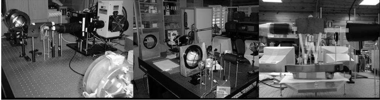
Fig. 4. Transmission assemblies: Left: for the camera, Center: The field lens and collimator, Right: Assembly and optical path for one of the folders.
