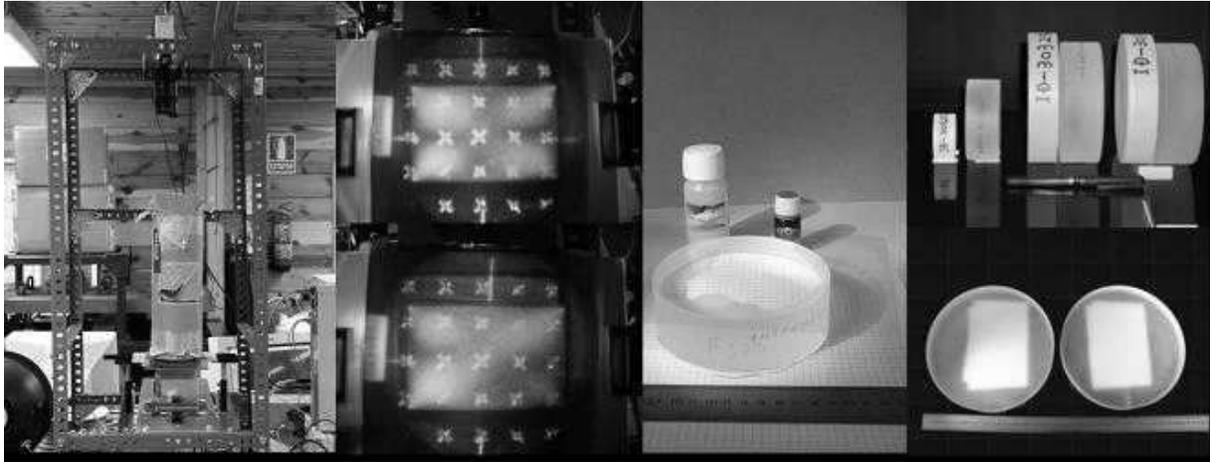
Fig. 2. Picture on the left shows the full assembly for the birefringence test. In the middle, some raw images of a FSL5 120x120x90 mm blank. Picture on the right shows a  $\text{CaF}_2$  blank while is being inspected using glycerin and the blanks of the camera (top right), collimator and field lens (bottom right).
