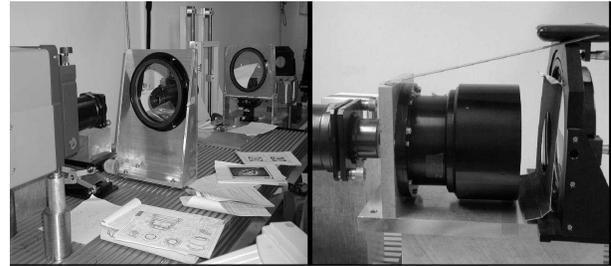
Fig. 3. Interferometric assemblies of field lens/collimator (left) and the camera (right) in SESO. All the WFE results were in specifications.
