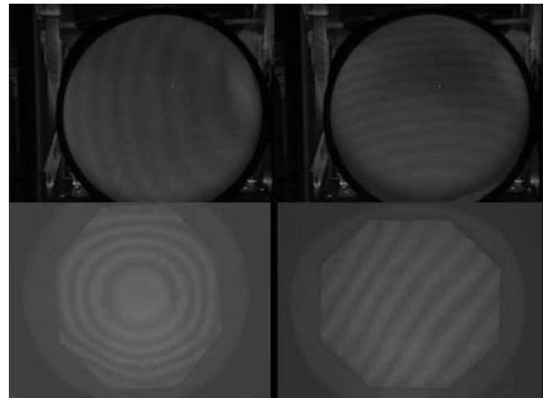
Fig. 8. Top, ZnSe prism with severe turned down edge that is nominally out of specification. Bottom, window interferogram. The flat surface (around  $\lambda/8$ ) was used to place the replica grating while the other side was cemented. This second surface was out of specification.
