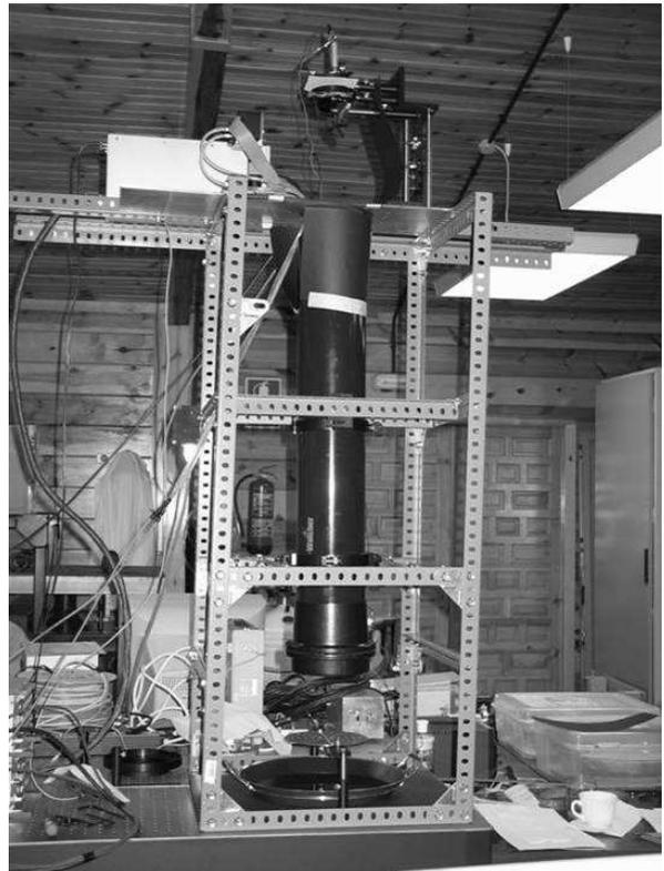
Fig. 6. Left, Hartmann assembly. The Hartmann had a beam of 150mm diameter and was placed vertically to have an oil surface at the bottom.
