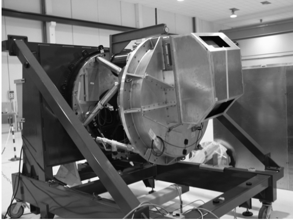
Fig. 2. ELMER on its test bench, testing the deflection of the whole instrument under self weight.
