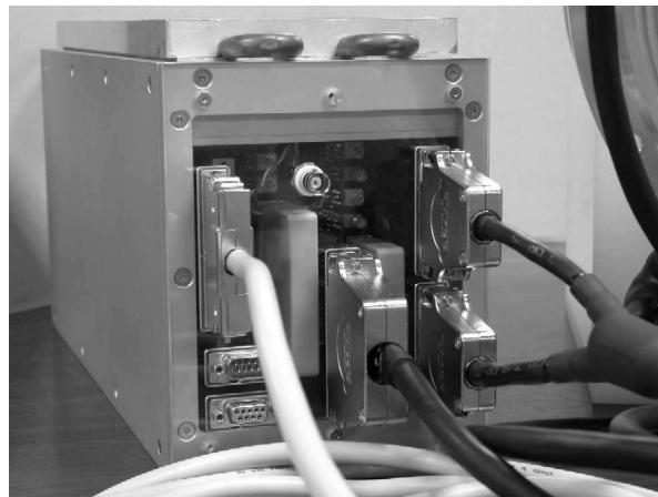
Fig. 5. SDSU-II controller for ELMER with external connectors. The custom prototype front plate has been made from plastic to verify the tracing of the internal cabling. In the final system a metal front plate will be used.
