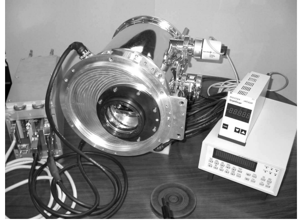
Fig. 1. ELMER CCD camera: LN 2 bath cryostat with CCD head and engineering flat window mounted (middle part), SDSU-II CCD controller (left), and Lakeshore 331 temperature controller and Pfeiffer TPG 261 vacuum gauge controller (right).
