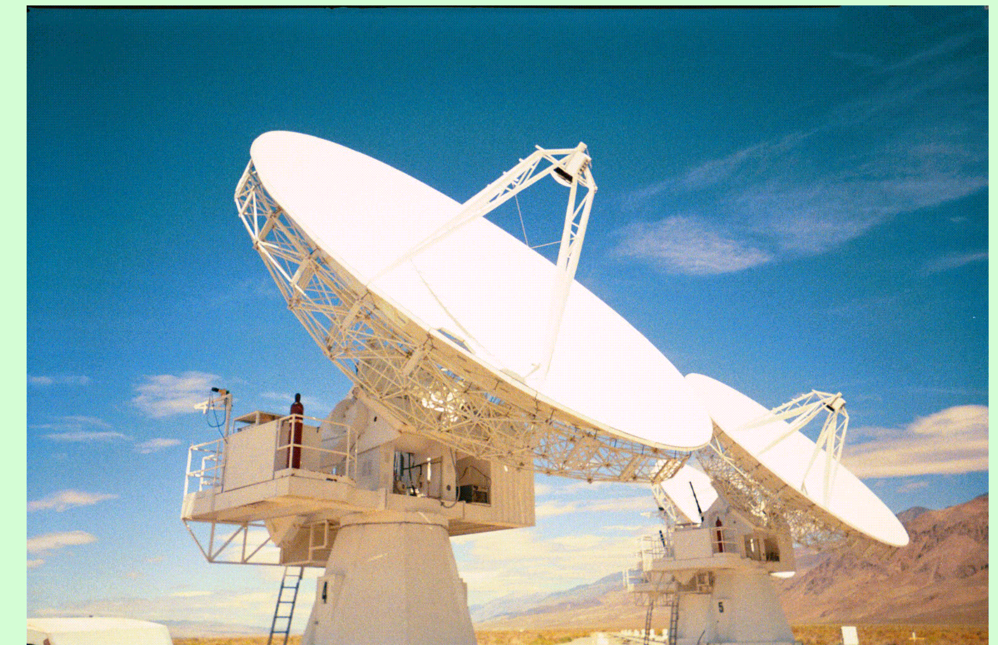
OVRO millimeter Array: 6 antennas, each 10.4m in diameter
