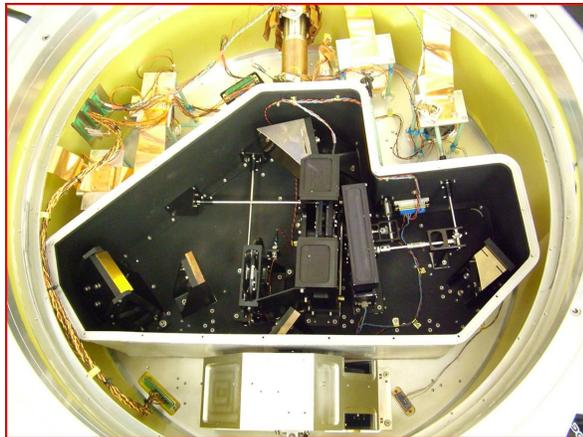
Fig. 1. Entrance window side of CanariCam, clearly showing two of the three off axis parabolic mirrors, three of the folding flat mirrors, the entrance aperture box and the filter and Lyot wheels.
