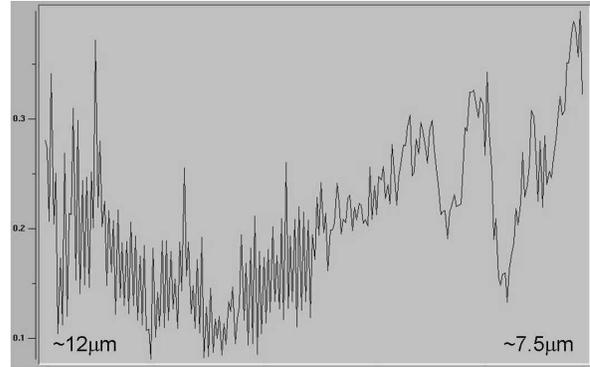
Fig. 4. The degree of polarization vs. wavelength in spectropolarimetry mode for a 0% polarized source.
