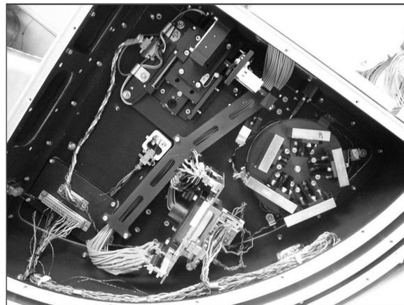
Fig. 2. Array side of CanariCam, clearly showing the grating turret (lower right), array (lower middle) and Wollaston prism slide (top middle).
