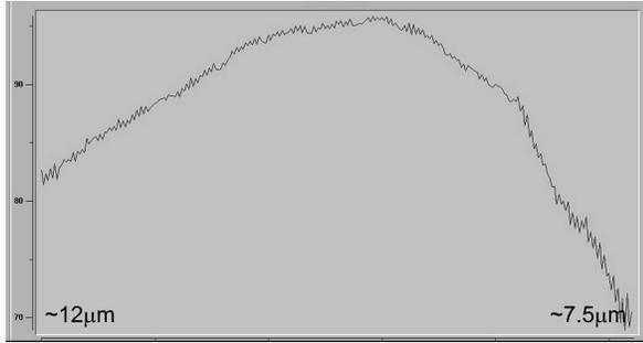
Fig. 3. The degree of polarization vs. wavelength in spectropolarimetry mode for a 100% polarized source.
