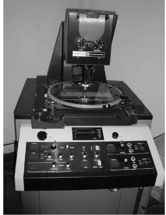
Fig. 2. PDS microdensitometer is the ideal instrument for digitize plates.
