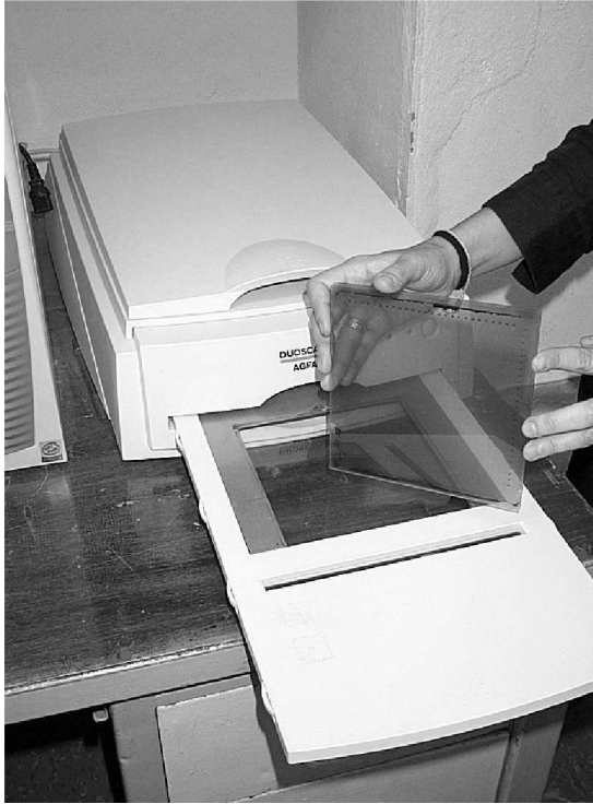
Fig. 3. A commercial flatbed scanner has been used as alternative for a digital reproduction of plates. Carte du Ciel San Fernando plates have been digitized with excellent results.
