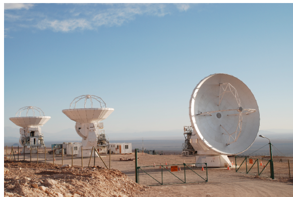
Fig. 4. A Mitsubishi antenna undergoing holographic surface measurements.
