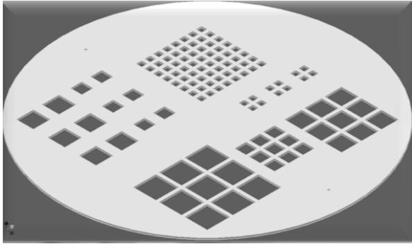
Fig. 2. 3D model for wafer micromachining structure.
