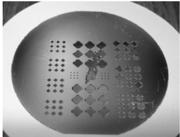
Fig. 4. Picture of  $45^\circ$  rotate masks wafer experimental micromachining results. All diaphragm support their own weight.
