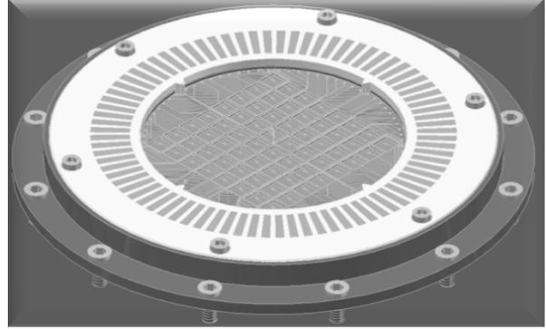
Fig. 7. 3D model for 8 × 8 elements bolometer, Copper base and Teflon<sup>®</sup> printed circuit board for electrical connections.
