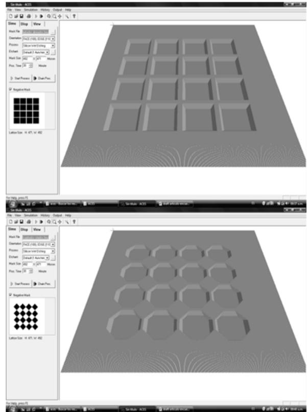
Fig. 3.  $4 \times 4$  elements micro machined array simulation made with ACES with (110) planes parallel to masks (up) and rotated  $45^\circ$  respect same plane (bottom).
