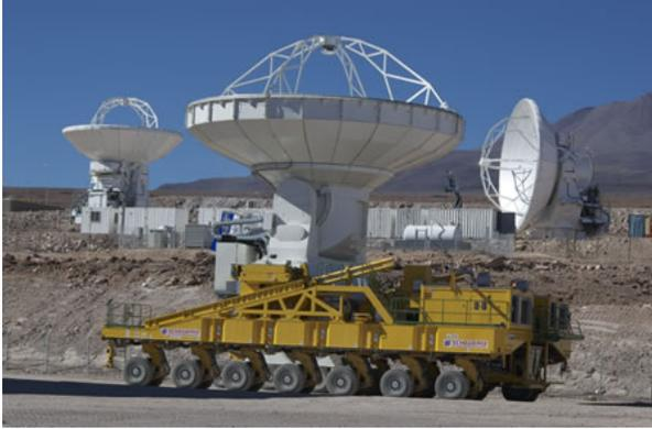
Fig. 1. One of the ALMA 12 m antennas being moved on a transporter at the mid-level ALMA facility (OSF, altitude 2900 m). The high site (AOS, at 5000 m) lies just over the ridge in the far distance.
