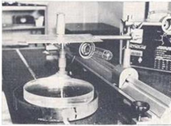
Fig. 4. Experimental arrangements for testing the primary mirror with the Ronchi test, and secondary mirror with the Newton fringes of the 84 cm Ritchey-Chrétien telescope.
