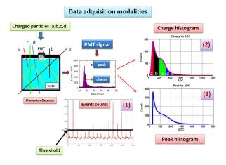
Fig. 2. High energy charged particles (a, b, c, d, e) produce Cherenkov Radiation in the water. The Cherenkov light fills the entire volume of water due to diffuse reflection on the tyvek. A light portion is collected by the PMT. The signal can be acdquiered as single events (1), charge (2) or peak histogram (3).
