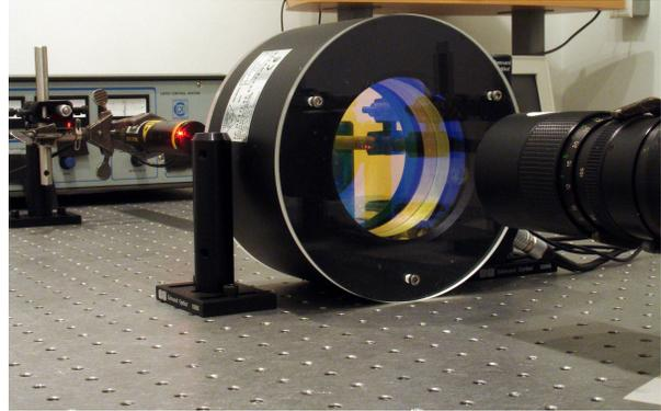
Fig. 1. NEFER scanning Fabry-Pérot interferometer characterization test at the Instituto de Astronomía laboratories.
