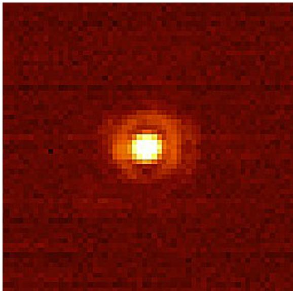
Fig. 1. A stellar image made with CanariCam during commissioning. This 1-s exposure at  $12.5 \mu\text{m}$  has a full-width at half-maximum (FWHM) intensity of about 0.3 arcsec, essentially the diffraction limit. Note the first Airy ring and a hint of the second.
