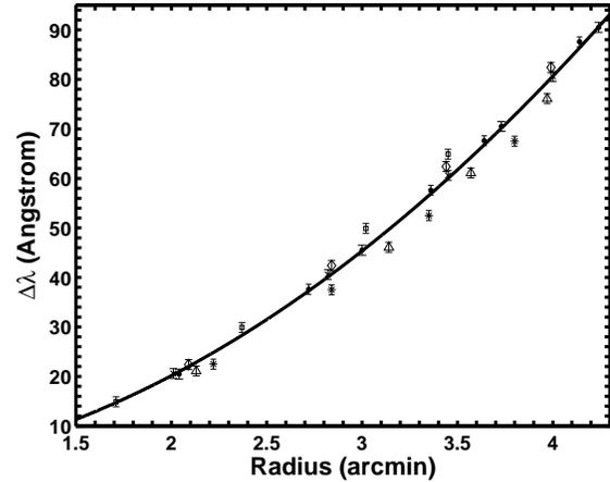
Fig. 2. Variation of the difference between the tunable filter central wavelength and the wavelength, versus distance to the optical centre, for the red tunable filter and for wavelengths ranging from 660 nm to 920 nm.
