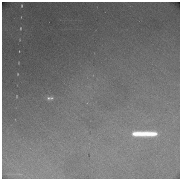
Fig. 4. Composition of the movement of the Argentine satellite Nahuel-1A and the Venezuelan Venesat1, both geostationary satellites, while the first one passes by the window of the second one, obtained from the observations corresponding to the nights of May 27 and 28, 2010. In the intermission there were maneuvers of the Venezuelan satellite and for this reason it appears like a double dot.
