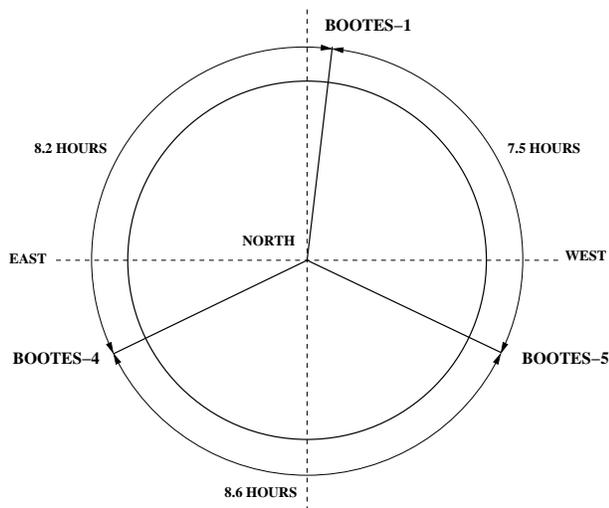
Fig. 1. Longitude separation between telescopes at the BOOTES-1, -4, & -5. The time separation between adjacent sites is shown.
