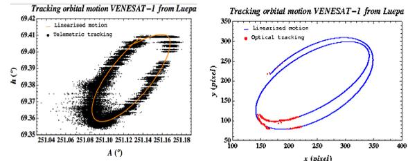
Fig. 5. Orbital motion projected on the horizontal plane (topocentric coordinates). Left plot represents telemetric tracking while right plot represents optical tracking where the vertical and horizontal axes correspond to Elevation and Azimuth.
