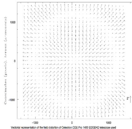
Fig. 2. A vectorial representation of the distortion introduced by the CGE PRO 14 00 EDGEHD telescope.
