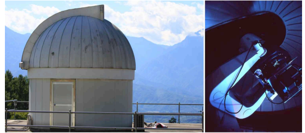
Fig. 1. MITSuME Akeno Observatory and its 50 cm quasi-Ritchey Chretien reflector.
