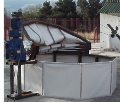
Fig. 1. The dome system designed for MASS-DIMM
