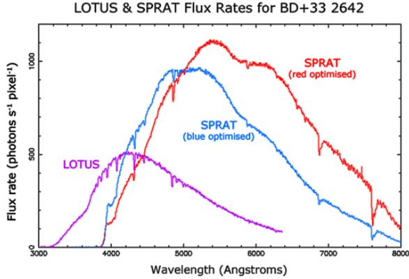
Fig. 2. Relative flux rates in photons per second per  $4.7\text{\AA}$  pixel from LOTUS and the blue and red optimized modes of SPRAT for the spectrophotometric standard star BD+33 2642.
