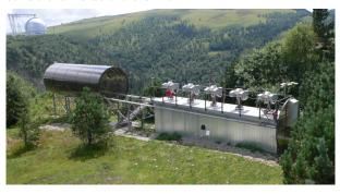
Fig. 2. Photo of the all 9 channels of MMT installed on 5 mounts in the single cylindrical dome, which is open at that moment. The russian 6-m telescope may be seen in the background.
