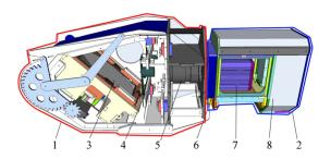
Fig. 1. Schematic view of a MMT channel. 1 – coelostat unit, 2 – camera unit, 3 – coelostat mirror which can rotate for  $\sim 10$  degrees around two axes, 4 – installable color and polarimetric filters, 5 – Canon EF85/1.2 objective, 6 – optical corrector, 7 – Andor Neo sCMOS detector, 8 – conditioner to keep stable environmental conditions inside the channel.
