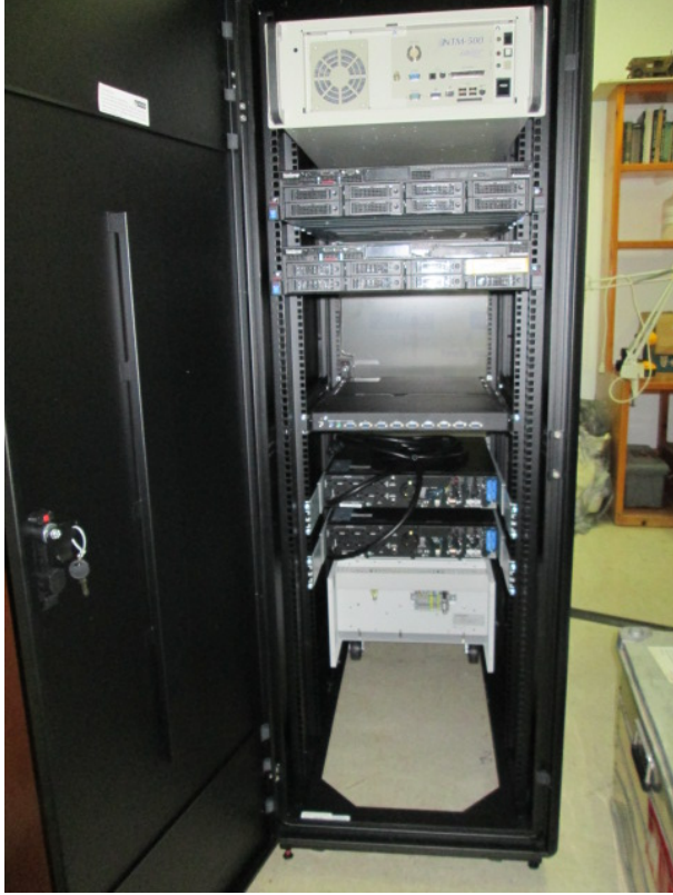
Fig. 4. BOOTES-5 Rack. From top to bottom are located: NTM-500 mount controller computer; server; backup server; keyboard and monitor (shutdown); UPS-A; UPS-B; and American-European voltage converter.
