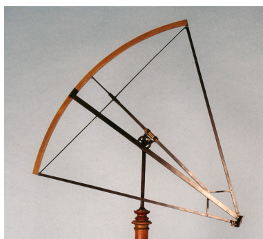
Fig. 4. A brass sextant of 1145 mm radius as used in Kassel from 1585 for producing the catalogue of 384 stars. The elegant metal construction is quite different from the massive wooden instrument of Tycho Brahe.
