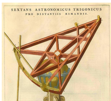
Fig. 3. Tycho Brahe's wooden sextant of 155 cm radius from about 1582.
