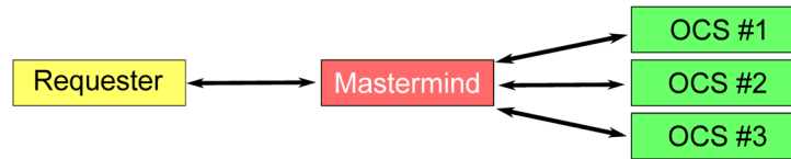
Fig. 6. Example for handling an observation request in a heterogeneous telescope network with a mastermind.
