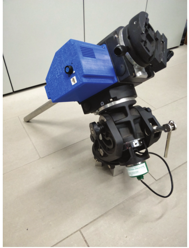
Fig. 3. Example of adaptation on a telescopes control system on a commercial AZEQ-G mount. Original DC motors were replaced by stepper motors powered by a customized Arduino shield.
