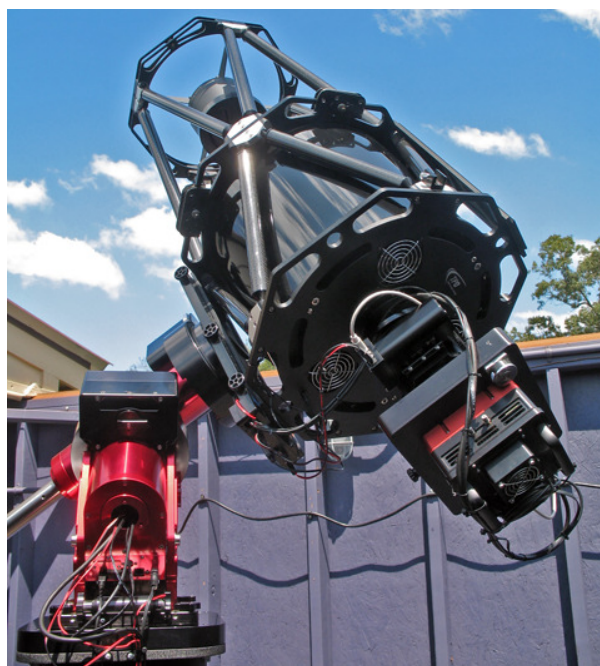
Fig. 3. Current telescope of Waffelow Creek Observatory: 0.356 RC telescope.
