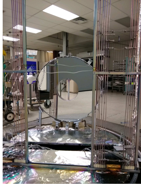
Fig. 4. Zadko Telescope primary mirror after re-coating.
