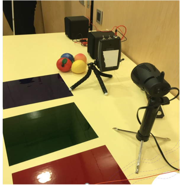
Fig. 3. This figure shows an Orchestar demo, using a light and 3 color filters - blue, green and red. The Orchestar is attached to a speaker to demonstrate the changing sound with color.
