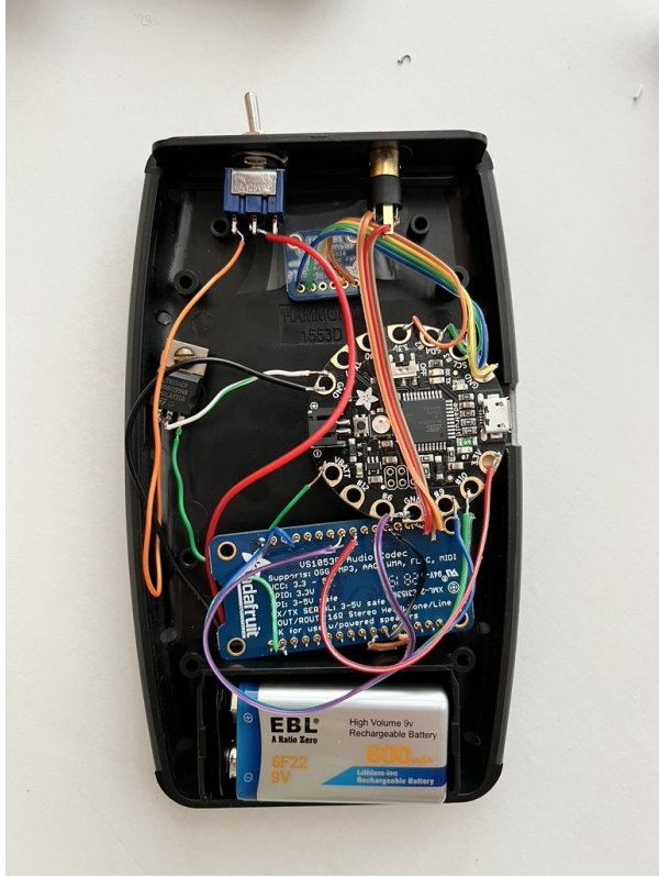
Fig. 2. This image shows a LightSound being built by the team in the Dominican Republic. In the image one can see the open chassis with the wires, battery and circuits.
