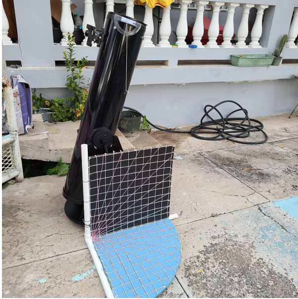
Fig. 5. This is an example of a setup in which the telescope is being aligned with a tactile protractor for declination and CARDIS for RA.
