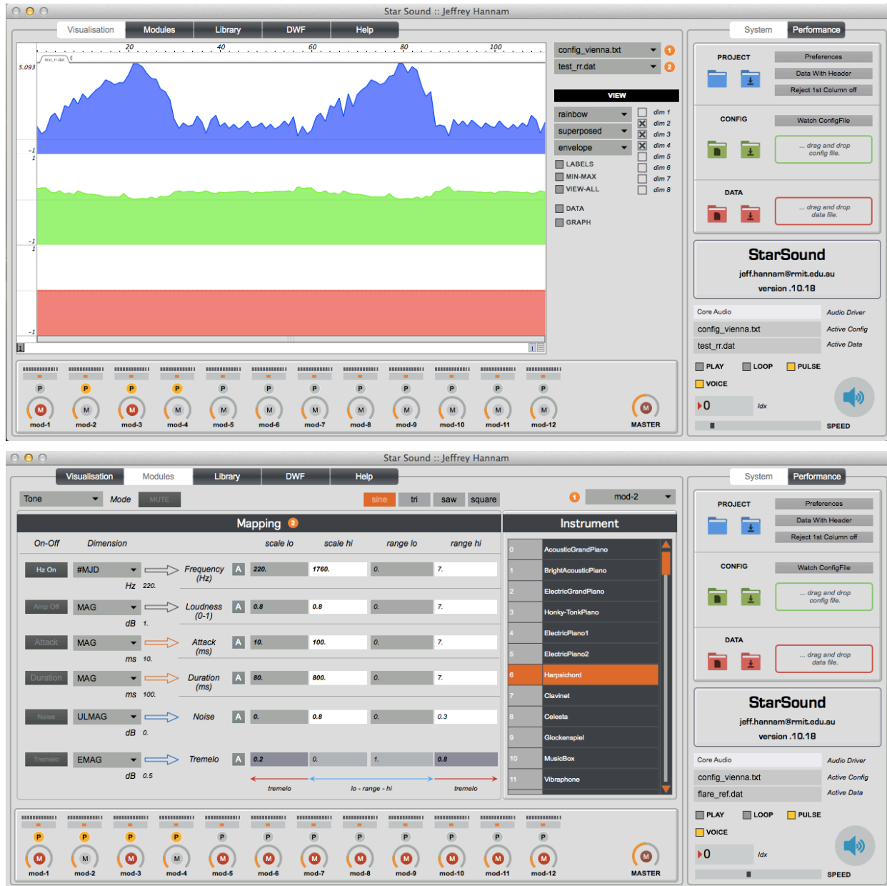
Fig. 1. Screenshots of the StarSound sonification software interface. ( Top ) The StarSound visualisation page. In this example the colour plot shows three discrete data channels being sonified (blue, green and red traces). To the right of the plot are dropdown menus for displaying and selecting configuration and data files, and controls for modifying visual features of the plot. Further right are controls for administering the sonification project, with a selection of features for controlling audio playback below. Along the bottom are pan (stereo) and mute controls for 12 separate channels ( Bottom ) The StarSound modules page for mapping data channels to sound and for setting the audible characteristics of the sonified data. The preferred sound generator (tone or MIDI instrument) is selected via a dropdown menu at the top. The data channel to be mapped is selected using the lefthand dropdown menus and sonified output is then tuned using the numeric entry fields to the right. Three other available interfaces (not shown) include a 'Library' for personal files, specific configurations for our 'DWF' research program, and a 'Help' interface.
