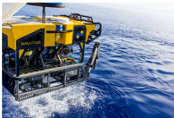
Fig. 1. The remote operation vehicle ROV SuBastian used for the exploration of the seabed and the collection of sediment cores during the 2018 oceanographic campaign.
