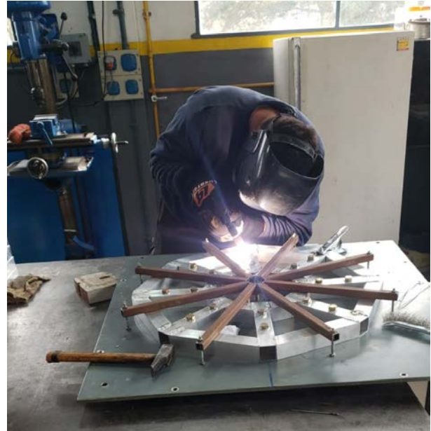
Fig. 18. Technician Nahuel Duarte soldering the aluminium hub for the MIA antenna assembly in the mechanical workshop.
