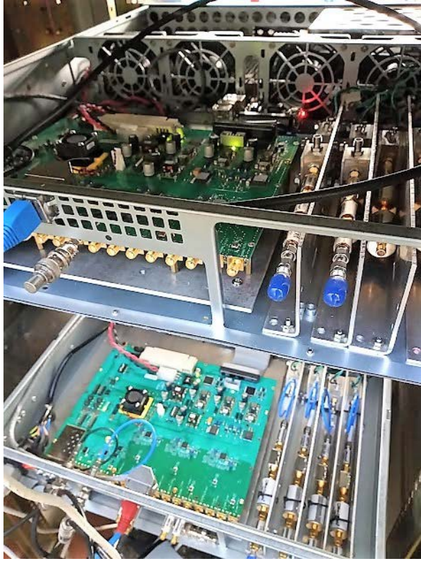
Fig. 14. Digital Back-End (DBE) for the Deep Space Antennas.
