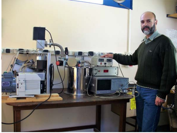
Fig. 22. Ing. Daniel Perilli standing next to the Dewars cryostat.
