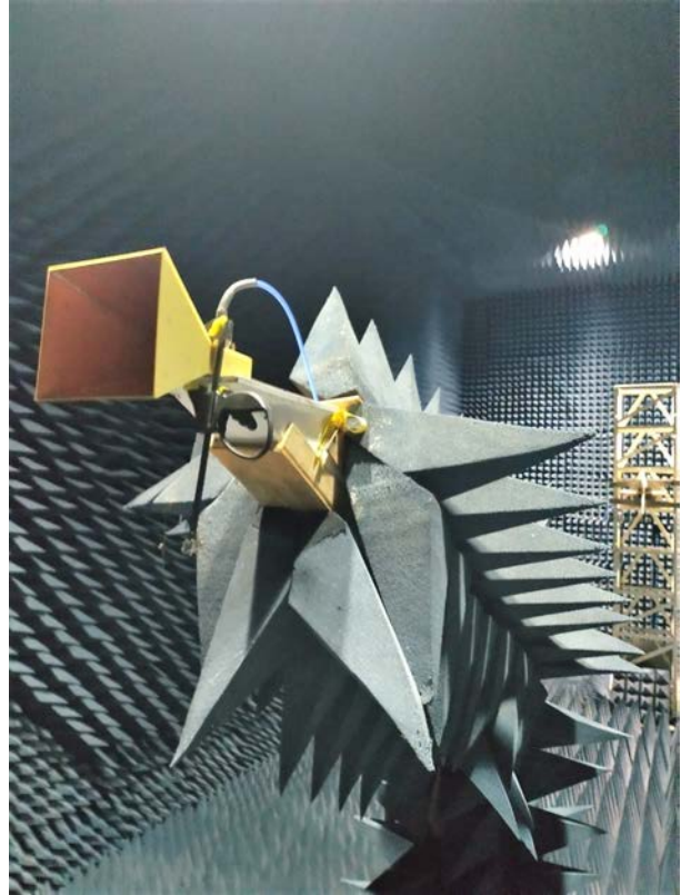
Fig. 21. Antenna characterization tests inside the anechoic chamber.
