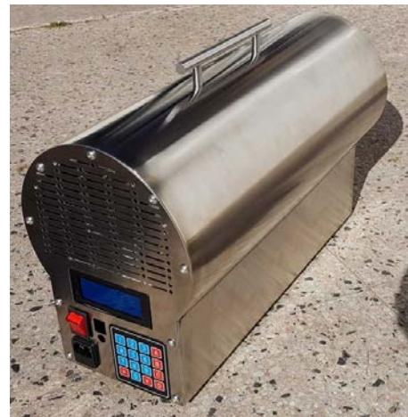
Fig. 11. Production model of the first ozone reactor to be used in public space during the COVID-19 pandemic.
