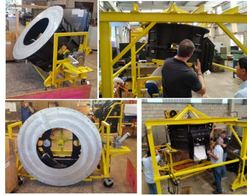
Fig. 8. CASS handling and integration in the Cab-CASS fixture.
