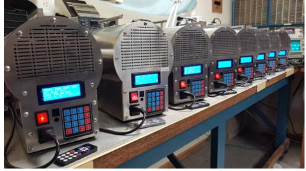
Fig. 25. Assembly line of ozone reactors for sterilization close spaces.
