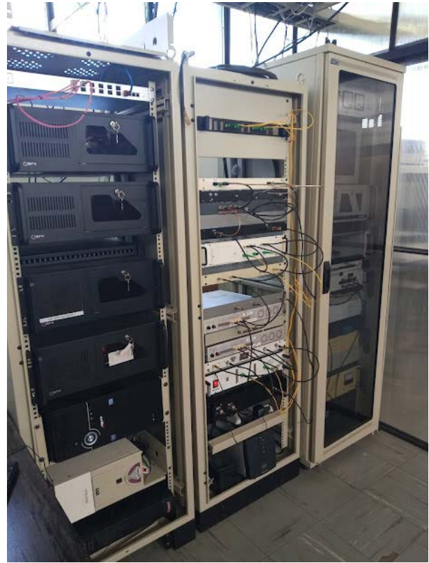
Fig. 22. Digital back-end based on ROACH boards developed by CASPER collaboration and storage in the control room of IAR's radio telescopes.
