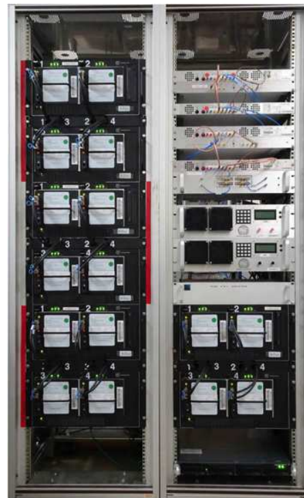
Fig. 10. EHT digital VLBI backend as installed at the Institut de Radioastronomie Millimétrique (IRAM) PV 30 m telescope in Spain. Right-hand side upper rack are located the four R2DBE units. Two block downconverters are installed near the middle, and the VLBI backend computer is mounted on the bottom right. The rack on the left and the lower portion of the rack on the right hold the four Mark 6 recorders with four disk modules each, providing a total of about 1 PB in data storage.
