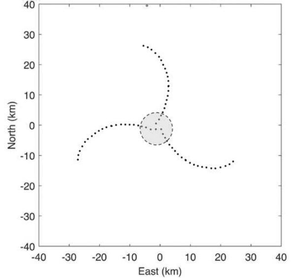
Fig. 2. Distribution of 64 MIA antennas on the Auger Observatory site assumed in this work, distances are in Km.
