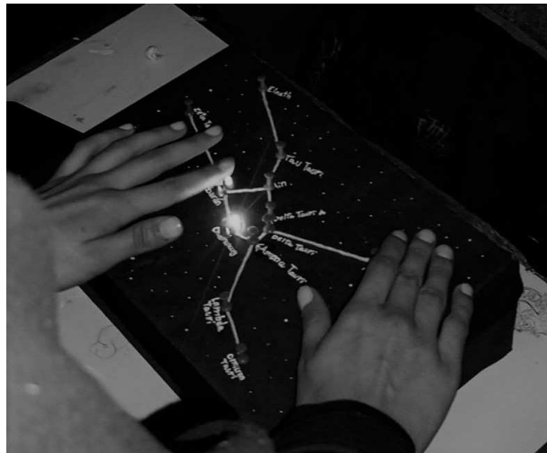
Fig. 2. A tour of the final model with the fingers. The blindfolded subject must 'finger-walk' through the constellation, pulsate on the selected stars and listen to the differences in volume and pitch. The circuitry is inside the box.
